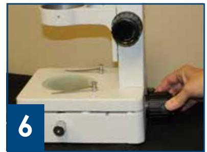
To use incident lighting, attach the upper illuminator bracket to the silver mounting block on the top of the light control unit. Insert the light assembly into the ring holder. Insert the plug at the end of the light assembly into the receptacle on the back of the light control unit. Plug the cord into the wall.
