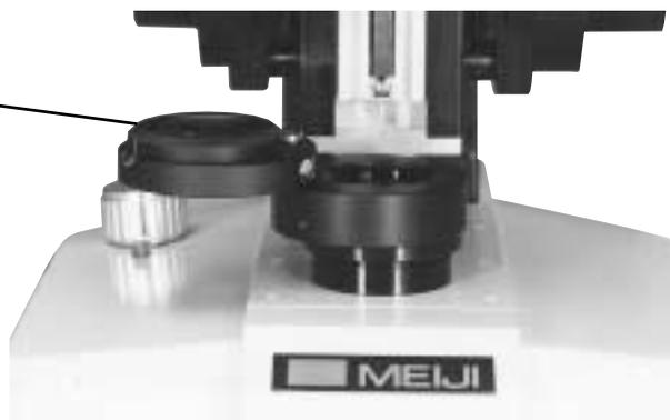
(The picture shows that substage polarizer is swung out.)
