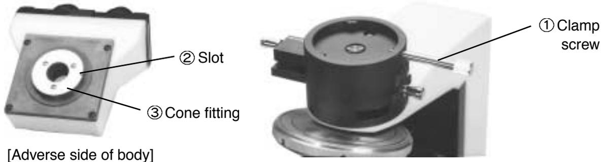
To mount the body, loosen the Clamp screw ① and insert the Cone fitting ③ of the body into the recess in the top of the limb and clamp it by the clamp screw.
