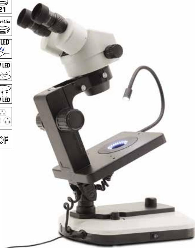
Binocular gemological stereomicroscopes for brightfield and darkfield applications with special side-emitting **LED** illumination ring for true darkfield illumination. Equipped also with an incident **LED** flexible arm and a diffusive **LED** disc for transmitted illumination. The instrument can be easily tilted horizontally for immersion analysis.
