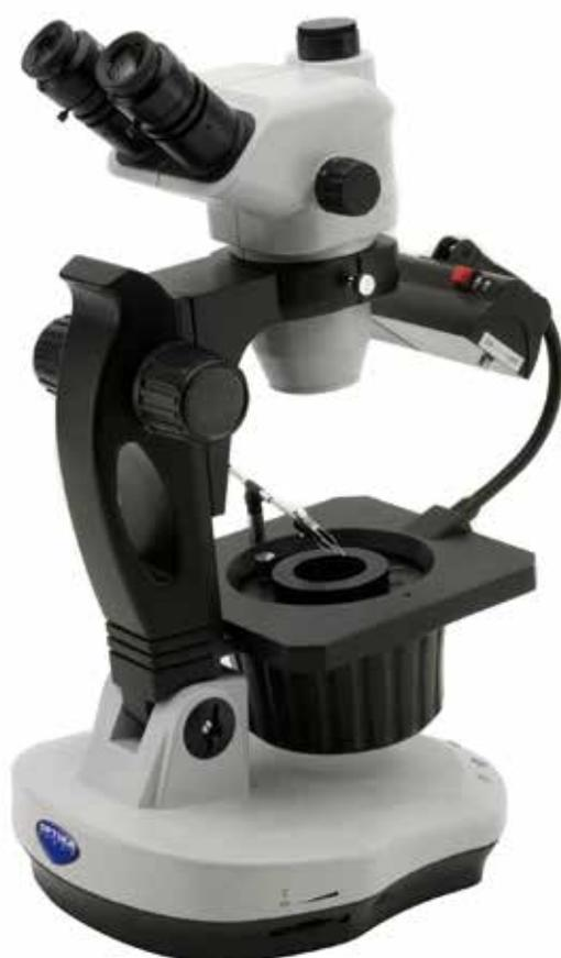
Trinocular gemological stereomicroscopes for brightfield and darkfield applications. The darkfield condenser uses a typical optical configuration, based on halogen illumination and a classic reflecting system. A flexible arm with a fluorescent tube simulates the color of daylight for accurate color grading. The stand can be inclined backward by 45° for to increase comfort and ergonomy.
