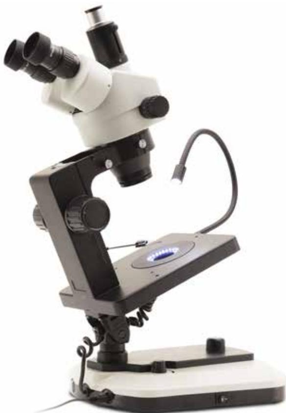
Trinocular gemological stereomicroscopes for brightfield and darkfield applications with special side-emitting **LED** illumination ring for true darkfield illumination. Equipped also with an incident **LED** flexible arm and a diffusive **LED** disc for transmitted illumination. The instrument can be easily tilted horizontally for immersion analysis.
