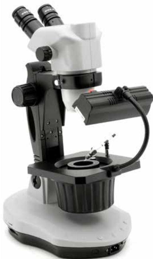
Binocular gemological stereomicroscopes for brightfield and darkfield applications. The darkfield condenser uses a typical optical configuration, based on halogen illumination and a classic reflecting system. A flexible arm with a fluorescent tube simulates the color of daylight for accurate color grading. The stand can be inclined backward by 45° for to increase comfort and ergonomy.
